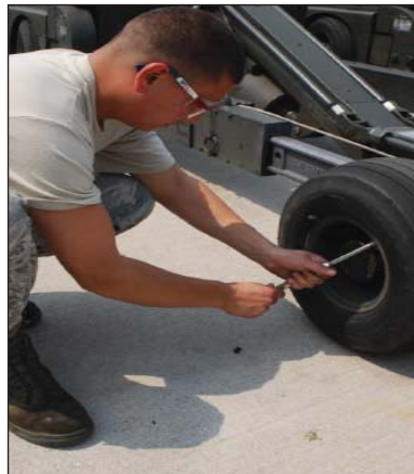
Senior Airman Isaac Amador checks the tire pressure on an MHU Bomblift during a routine service inspection.
