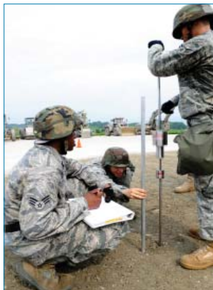
Senior Airman Christopher Davis, left, Airman 1st Class Jason Alfaro, center, and Airman 1st Class Chi Li test the compaction of a filled crater using a dynamic cone penetrometer at Jungwon Air Base, Republic of Korea, Aug. 19. The reading tells if the crater is sufficiently filled and compacted to withstand aircraft landings. Airmen Davis, Alfaro and Li are assigned to the 51st Civil Engineer Squadron here.
